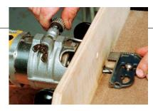
**Depth adjustment.**The depth of the cut is controlled using the adjustment gauge on the router.
