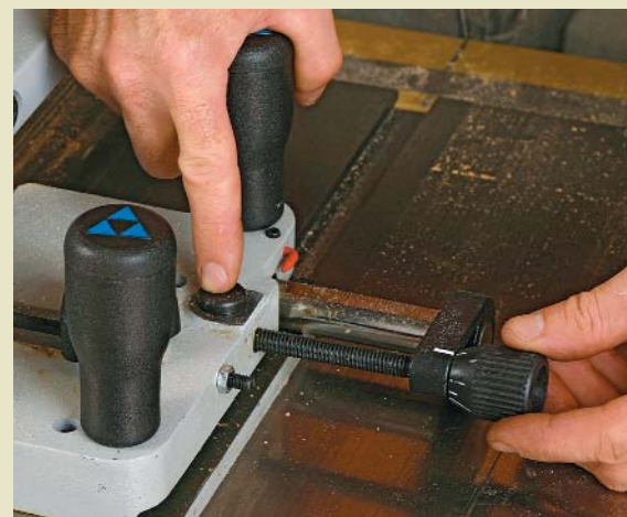
Side-to-side adjustment. When it came to establishing the tenon width, the Delta proved easiest to use—just push a release button, slide the main fence sideways, and then fine-tune the location with the micro-adjustment dial.
