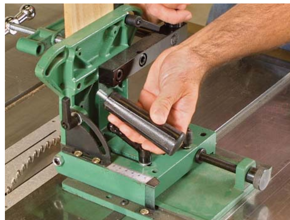
Adjustable handle. Most of the jigs offer at least one alternate handle position.
