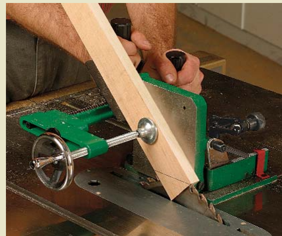
Front-to-back tilt adjustment. Using the secondary fence, each jig allows the workpiece to tilt backward up to 45°.
