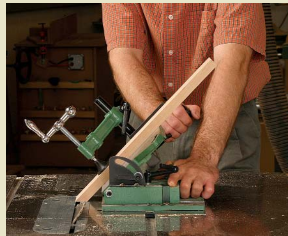
Side-tilt adjustment. The jigs have a main fence that can be tilted left up to 18°, 24°, or 45°, depending on the manufacturer.
