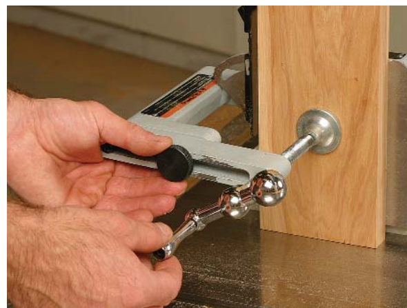
Knob makes adjustments easier. When wide stock dictates that the clamp arm has to be slid forward, Purdy preferred the jigs that locked the arm with a knob (shown) over those that called for an Allen wrench.
